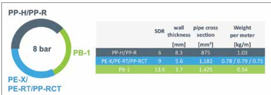
Figure 1 ... PB-1 is the material with the highest SDR class.
