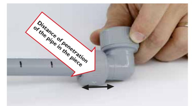
Push the pipe firmly into the fitting until the end reaches the line marked by the felt-tip pen. Thus, with a quick look we check that it is properly joined.
