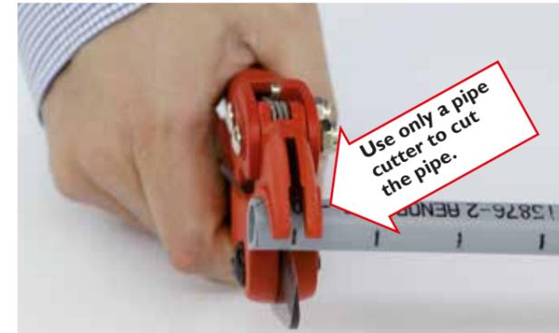
Use only a pipe cutter to cut the pipe. Never use a hacksaw. To ensure a clean, square cut, rotate the pipe whilst maintaining pressure on the cutter until the pipe is severed.
