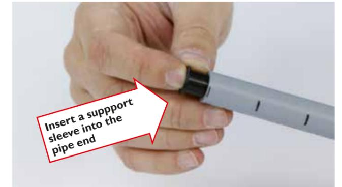
Insert a support sleeve into the pipe end. DO NOT FORGET this step, as otherwise it might come out of the fitting.
